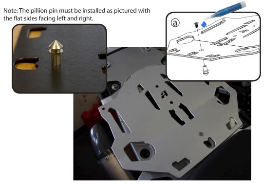
(a) Install the male locator pin to the pillion rack using the provided M6 flat head, use a drop of thread locker and tighten completely. (b) install the pillion rack the same way you would Install or remove your passenger seat.
