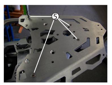
Add rear rack and use the M4 allen driver to install the (4) M6 x 35 flat head screws. Tighten them all the way down.
