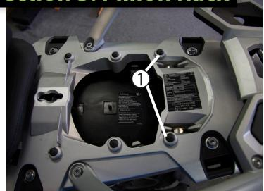
Using your BMW key, remove the pillion (passenger) seat. Also complete step #2 in section 2 to remove the OEM luggage rack if you have not already. Remove (2) rear oem rubber bumpers and save them for later in case you would like to run the passener seat again. Use lubrication to re-install the rubber bumpers.
