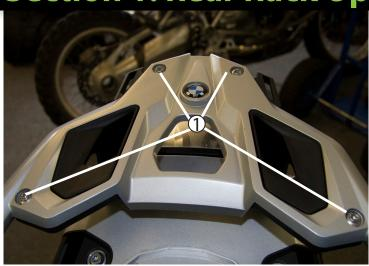
Remove (4) OEM screws using a T30 Torx driver. Save these screws but they are not needed to finish this installation.
