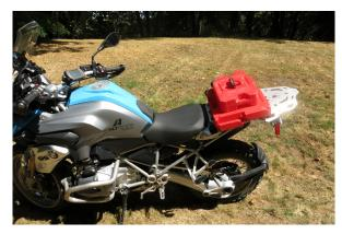
AltRider Luggage Rack System - R113-P-4002 **RotopaX Locking Mount** - ROTO-1-7111 **Rotopax Mount Extension** - ROTO-1-7112 RotopaX 1 Gallon Gasoline Pack - ROTO-1-7100 RotopaX 2 Gallon Gasoline Pack - ROTO-1-7115
