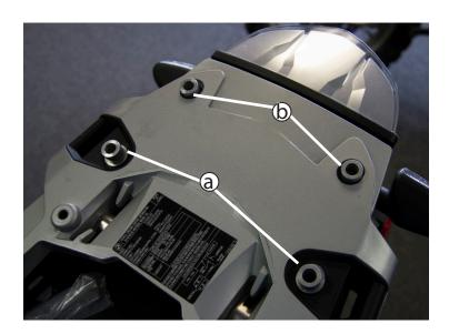
Place the (2) 11mm spacers in the front (a) and the (2) 12.7mm spacers (b) in the rear. TIP: to hold the spacers from sliding around use a small dab of grease on the bottom of each spacer.
