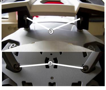
Place the pillion rack and lock into place. (a)Using a T40 Torx driver install the (2) OEM T40 x 40 mm bolts from step 2 in section 2, do not tighten all the way. (b)Using a T40 Torx driver install the (2) OEM T40 x 40 mm bolts from step 2 in section 2 into the rear mounting position of the tail rack. Torque all (4) fasteners to 10 nm.
