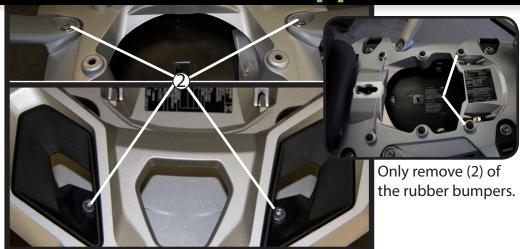
Remove the BMW upper rear plastic rack with grab rails (Section 2: steps 1 and 2). Install pillion rack per instructions (section 3).
