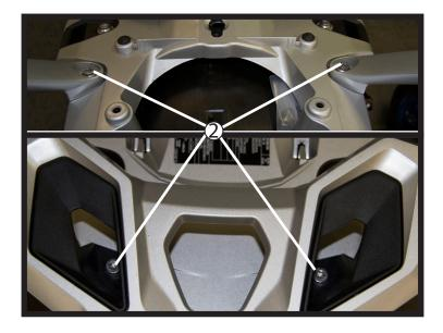
Remove (4) OEM bolts with a T40 Torx driver. Save these bolts but they will not be used to finish this installation. Remove the oem luggage rack and store for later usage.
