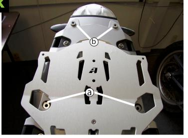
Place the (2) 15mm spacers in position (a) inside front mount holes for grab handles. Place the 11mm spacers in position (b) inside rear mount holes of tail rack.
