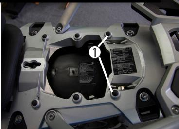
Using your BMW key, remove the pillion (passenger) seat. Also complete step #2 in section 2 to remove the OEM luggage rack if you have not already. Remove (2) rear oem rubber bumpers and save them for later in case you would like to run the passener seat again. Use lubrication to re-install.
