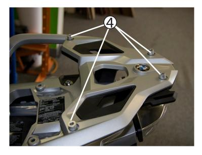
Add the (4) provided 15mm spacers with slanted end facing the front of the bike.
