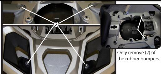
NOTE: YOU MUST HAVE THE ORDERED THE REAR RACK OR FULL SYSTEM TO BE ABLE TO COMPLETE THIS SECTION. Remove the BMW upper rear plastic rack with grab rails (Section 2: steps 1 and 2). Install pillion rack per instructions (section 3).
