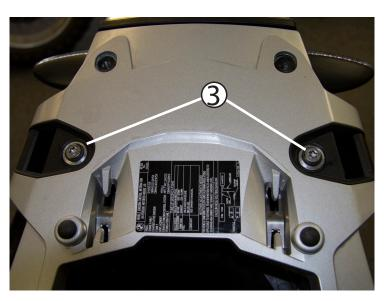
3 Remove the (2) remaining OEM bolts with a T40 Torx driver. Put these in storage for later usage. You will not need them to complete this installation. Keep the OEM washers in place.
