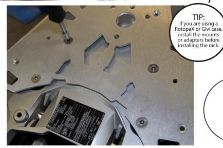
Pillion rack is VERY TIGHT when installed and removed for the first couple of times. This is an intentional part of our design and is meant to prevent a sloppy fitment and rattling in the future. The installation and removal process improves over time.
