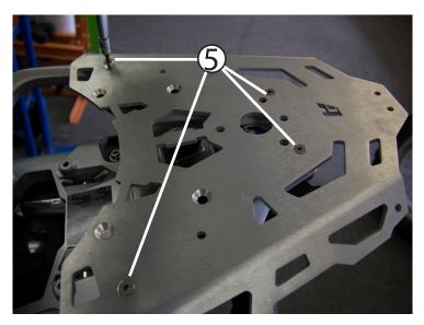
3 Add rear rack and use the M4 allen driver to install the (4) M6 x 35 flat head screws. Tighten them all the way down.
