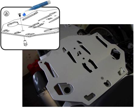
(a) Install the male locator pin to the pillion rack using the provided M6 flat head, use a drop of thread locker and tighten completely. (b) install the pillion rack the same way you would Install or remove your passenger seat.
