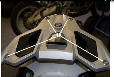
Remove (4) OEM screws using a T30 Torx driver. Save these screws but they are not needed to finish this installation.
