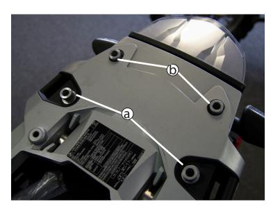
Place the (2) 11mm spacers in the front (a) and the (2) 15mm spacers (b) in the rear. TIP: to hold the spacers from sliding around use a small dab of grease on the bottom of each spacer.
