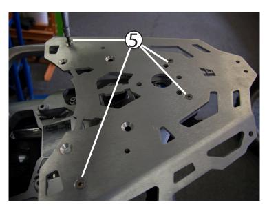
Add rear rack and use the M4 allen driver to install the (4) M6 x 35 flat head screws. Tighten them all the way down.
