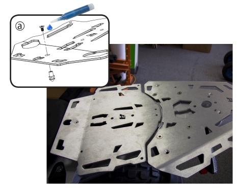
(a) Install the male locator pin to the pillion rack using the provided M6 flat head, use a drop of thread locker and tighten completely. (b) install the pillion rack the same way you would Install or remove your passenger seat.
