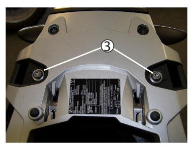
Remove the (2) remaining OEM bolts with a T40 Torx driver. Put these in storage for later usage. You will not need them to complete this installation. Keep the OEM washers in place.
