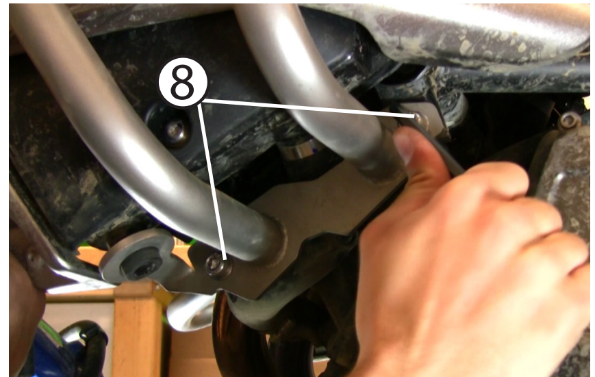
⑧ Using a 6mm allen tool, finish tightening the (2) provided fasteners down on the left and right side mount brackets.
