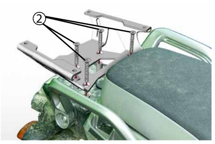
Using a 5mm allen tool, assemble the luggage rack onto the tail of the bike as shown. The order of assembly should go: mount points - provided spacers - mounting bracket - M8 fasteners. Note that the two longer standoffs go closest to the seat.
