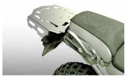
The AltRider luggage rack can also be configured as shown. You'll need to remove the grab handles to use the rack in this configuration. This configuration puts the rack level with the cargo platform under the pillion seat.
