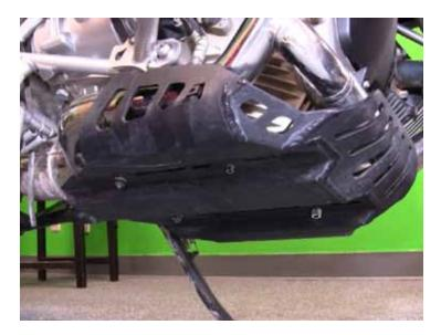
8 Your Skid Plate should look like this! Make certain your fasteners are all tightened to the MFG torque spec. After 100 miles of riding, check the fasteners again to make sure all is well.
