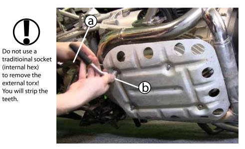
(a) Using an 18mm spanner, hold the vibration isolation mounts while (b) using the 13mm socket and a ratchet to loosen and remove the 2 rear nuts. (your hardware may vary)
