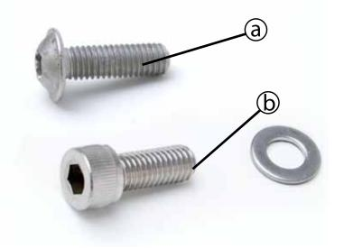
The other OEM front fastener (a) is a 6 x 20mm torx head. This 3 fastener is too long, and so we provide (b) a 6 x 12 cap head screw with a washer. You'll use a 5 allen key to tighten this.
