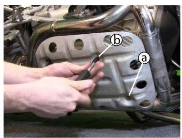
(a) Use an E10 socket to remove the large external torx fastener then (b) use an E8 socket to remove the smaller external torx fastener. Make certain that
