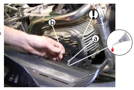
(a) hold the supplied M8 fastener (and washer) in place and (b) slide the aluminum spacer over it, then put the skid plate on and start the threads with your finger. (use thread locker!!)
