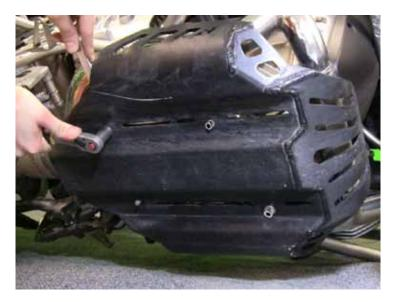
(a) Use a 21mm spanner to hold the vibration isolation mount while you, (b) tighten the 13mm nut. Tighten the M8 and the 13mm nuts to the MFG torque spec.
