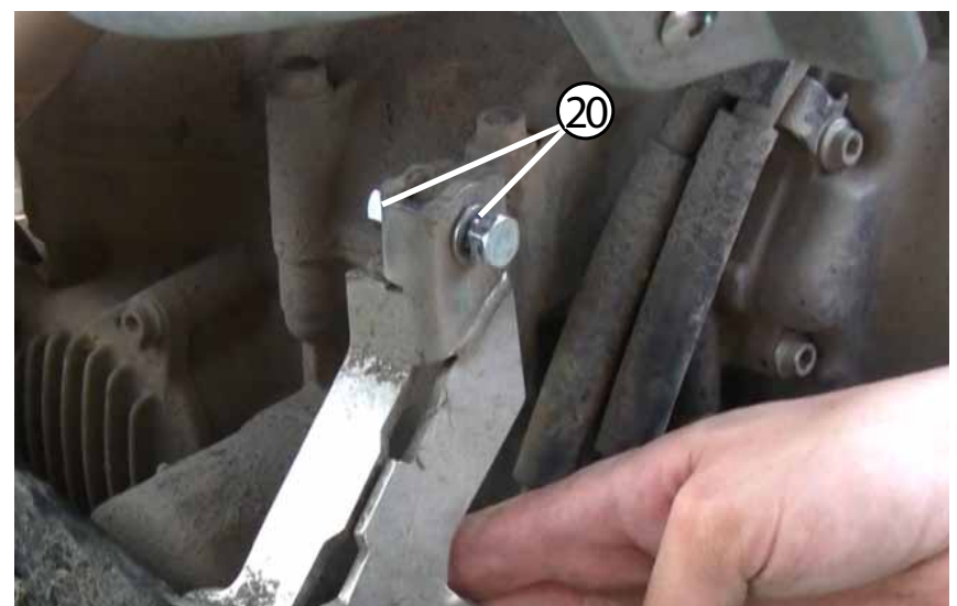
20 Last, you will tighten this bolt using a 13mm socket and 13mm wrench.
