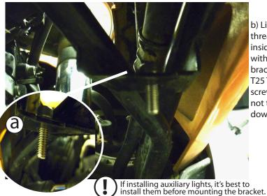
Using the T25 Torx socket, remove the (2) T 25 Torx fasteners from the front beak. Insert (2) M6x16 socket head cap fasteners and (2) M6 washers into the front subframe. See image (a).
