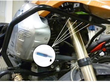
Rest the upper crash bar onto the existing lower crash bar assembly. Use a few drops of threadlockerand and start the (4) M6 x 35 socket head cap fasteners with (4) M6 washers into the upper bracket. All bar fasteners should be left loose.
