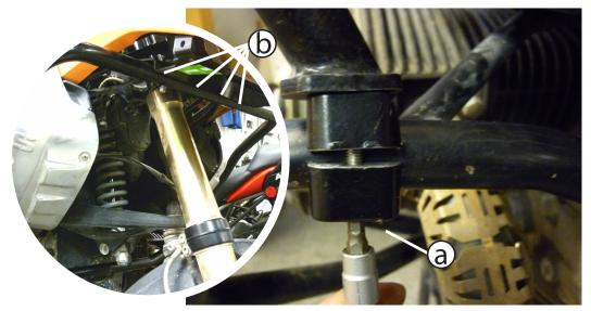
(a) Now slowly tighten both sets of clamps, alternating between front and rear screws so the clamps compress evenly. b) Go back and tighten the (4) M6 upper bar screws.
