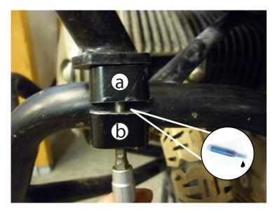
Slide the top clamp (a) under the upper crash bar mount. Apply a few drops of threadlocker to the (4) M6 x 35 socket head cap fasteners and lightly install with M6 washers into the lower clamp (b). Install from the bottom. On both sides, just give a few turns for loose fitment of the bar fasteners for now. Be careful when aligning the fasteners to avoid crossthreading.
