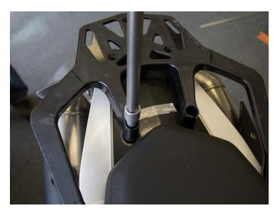
Using a T45 driver, remove the (2) OEM bolts. Save these bolts but you will not need them to complete this installation. ATTN: If installing RotopaX remove OEM rack first to make installation easier.
