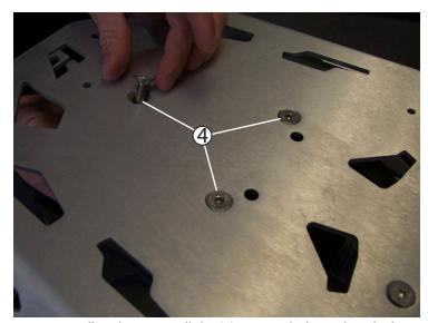
Using an M5 allen driver, install the (3) M8 x 25 bolts and M8 lock nuts. Hold the nut inplace from the bottom and tighten the bolt, the nut pocket will keep the nut from spinning. Go back and torque all (5) M8 bolts to 10 nm of torque.
