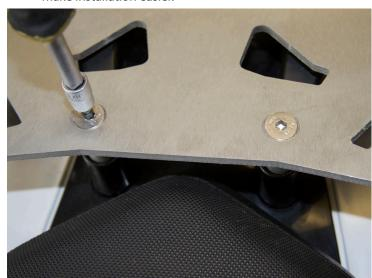
Place rack and install the (2) M8 x 90 bolts using a M5 allen driver. Do not tighten all the way.
