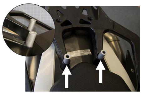
Place the (2) spacers as shown. Make sure the slanted end of the spacer is facing up and towards the front of the bike.
