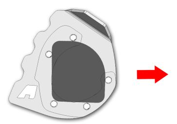
The arrow indicated should point toward the front of your bike. Adjust appropriately then check for intereference. Then you can tighten the fasteners!
