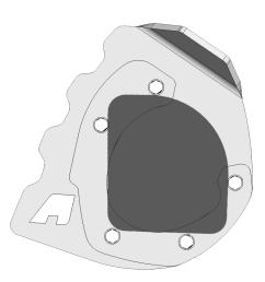
2 Looking down on the top of the large sidestand foot assembly, place the foot so that it is aligned as shown. Once in place, rotate the assembly so that it fits as indicated in step 3.
