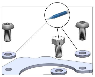
Apply one drop of Loctite to the last couple threads on all of the fasteners, then assemble the large sidestand foot on to your sidestand (indicated in step2).
