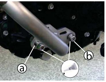
Using your fingers, insert the a) M8 x 40 w/washer and the b) M8 x 25 w/washer after using thread locker on the last couple of threads. Just a few turns for now, do not tighten these yet!
