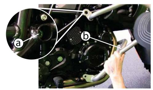
a) Using a T-50 torx bit, remove the upper motor mount bolt, an aluminum spacer will drop out, don't lose it.
