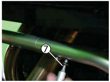
Using a 4mm allen bit, insert the remaining (2) M6 x 20 flat head screws. Tighten these down, as well as the (2) that you put in for step one. Be careful when inserting these, you are threading into aluminum. If it feels wrong, it probably is!
