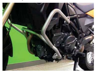
Now go back and tighten all of the remaining bolts. The (2) motor mounts, the (2) M8s on the right hand side, lower mount plate. And the (2) M8s on the left hand side, lower mount plate. Check all bolts after 100 miles of riding!!
