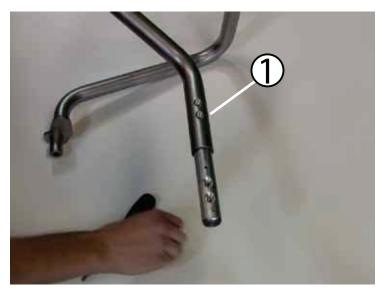
Insert the billet connecting rod into the riders right side crash bar so that the counter-sunk holes line up. Using your fingers, insert (2) of the M6 flat head screws. Just a few turns should do. Do not tighten these down yet!
