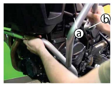
a) Remove the upper motor mount bolt on the left side (there won't be a spacer this time). b) Slide the left side crash bar on, connecter first, then into the upper frame tube.
