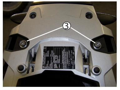
Remove the (2) remaining OEM bolts with a T40 Torx driver. Put these in storage for later usage. You will not need them to complete this installation. Keep the OEM washers in place.
