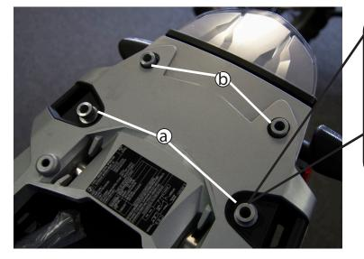
For the spacers called out as (a) in the image to the left: If you have a rack system installed which uses these two mount locations, you will need a 6mm spacer or (4) M8 washers will work insted of the provided spacers.
