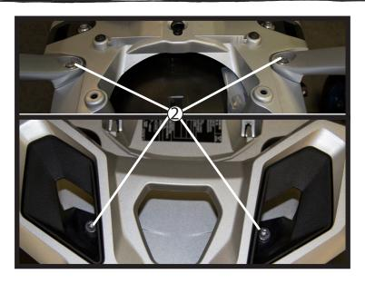
Remove (4) OEM bolts with a T40 Torx driver. Save these bolts but they will not be used to finish this installation. Remove the oem luggage rack and store for later usage.
