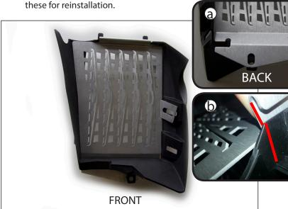
Fit each radiator guard into its respective shroud like pictured about. Make note of how they fit together be examining the shot of the assembly from behind (a) and where the radiator guard clips on to the top. If unsure how to line guard up to shroud, use diagram (b) and line up the two red lines.
