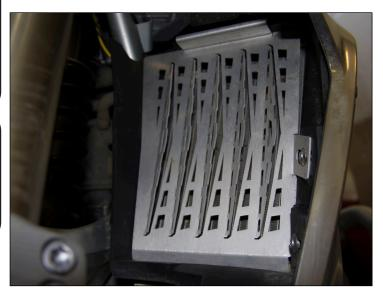
(4) Reinstall the shrouds with the radiator guards installed on them. Start by inserting the locator pins on the top of the radiator shroud. Reinstall the same (3) OEM screws on each side.
