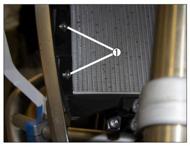
Using a T25 driver, remove the (3) oem screws holding the shroud over the radiator on each side (6 total screws). Save these for reinstallation.
