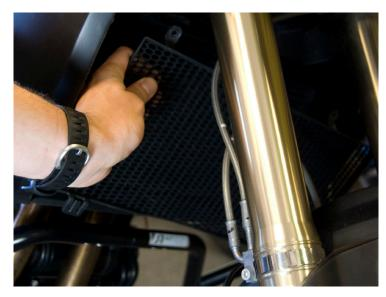
If installing radiator guard on 2013 and newer F 800 GS, skip to step 5. The OEM guard should come right out at this point. Rotate it forward then lift up on it slightly.
