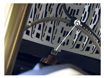
6 2013 and Newer F 800 GS: Install provided M5 screw, and washer and OEM nut to bottom mount using a M3 allen driver and 8mm wrench. All other models re-install the OEM screw and nut using a T25 driver and 8mm wrench.
