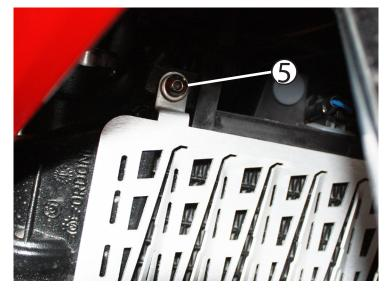
(5) Using your M3 allen driver, install the radiator guard starting with the (2) upper mounts. Install (1) M5 screw and washer on each side. On the 2013 and newer F 800 GS or the radiator guard simply fits over the existing plastic and you must install the (2) provided plastic spacers on top of the OEM plastic guard but under the AltRider radiator guard. If you have an F700GS or F800R you must also use the provided plastic spacers.
