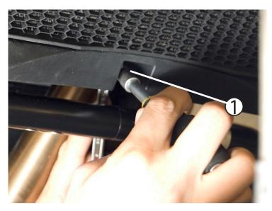
① Using a T25 tool and an 8mm wrench, remove the fastener in the bottom center, under the OEM radiator guard.
