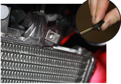
(4) If F 650 / 700 GS or F 800 R continue, if F 800 GS skip to step 5. Install the (2) M5 fender clips to the radiator top of the housing, (1) on each side. The clips will have to be slowly worked into place and will not install without resitance so take you time. If you cannot get them into place you can open up the clips slightly using a flat head screw driver.
