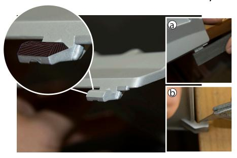
Remove tailbox lid. Using a file (a) or using a box knife (b), shave off the small bump on each tab of the tail box lid. This will allow for easier removal when the luggage rack is installed.
