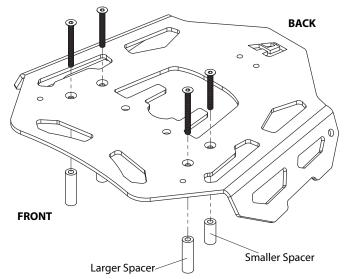
(3) Install luggage rack, spacers and screws. Start with the rear spacers and screws (smaller screws and spacers) and finish with the front spacers and screws. Tighten all (4) screws completely with M4 allen driver.
