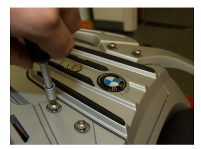
Using your T30 driver, remove the (4) T30 screws and set aside. You will not be reinstalling these screws.
