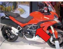
2. Remove the vacuum screw and replace it with the M6 spigot (part 6) re-using the original washer.
