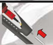
areas on the swingarm. Use self adhesive clips (part 13) to route delivery tubing. Route delivery tubing (part 14) neatly towards the RMV and secure to frame sections or similar using the cable ties (part 9). Trim to length and push firmly onto the spigot at the bottom of
