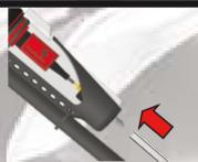
3. Clean the swingarm, then using the IPA wipe (part 18) degrease 2 small areas on the swingarm. Use self adhesive clips (part 13) to route delivery tubing. Route delivery tubing (part 14) neatly towards the RMV and secure to frame sections or similar using the cable ties (part 9). Trim to length and push firmly onto the spigot at the bottom of the RMV.
