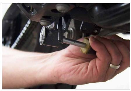
1 Push out the rubber plugs currently in the center stand mounts.
