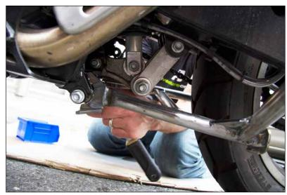
Using a 17mm socket and a 8mm hex driver, tighten the bolts into the nylon locking nuts to secure the stand. DO NOT OVER TIGHTEN, you need to leave enough play so that the center stand can move freely. Tighten to 41nm and then test the action.
