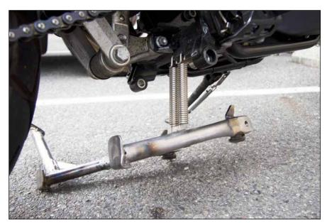
3 Hook the springs on to the two holes of the metal tab. Let the center stand hang here.
