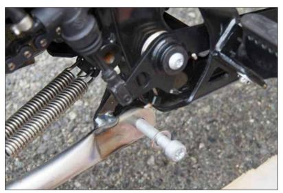
Insert both of the M10 x 60 hex cap bolts with the washers positioned as shown above. Sliding the bolts into place will hold the center stand in position. After both bolts are in place, slide one of the washers over the threaded end of each bolt.
