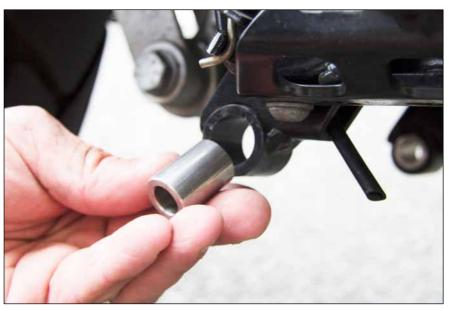
Grease the two aluminum bushings inside and outside. Slide them in to the mounts on both sides. Use enough grease so that it will hold the bushings in place.
