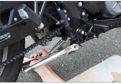
Have your fasteners accessible. Using the frame and right mount as a leverage point, push the left side mounting tab up to align it with the left mount on the bike. Both mounting positions are to the RIGHT of the mounts.
