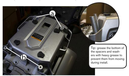
Place spacers, short spacers(a) in the back and tall spacers(b) at the front. Make sure that the front spacers(b) are at the correct angle.
