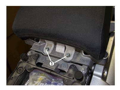
Remove the riders seat. Using an M5 allen remove the pillion seat mount screws and remove the pillion seat. Now replace the (2) OEM pillion mount screws. Torque to 10nm.
