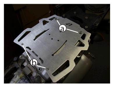
Install pillion rack and screws, short screws (a) in the rear and longer screws (b) in the front. Tighten using an M4 allen driver and torque to 10nm.
