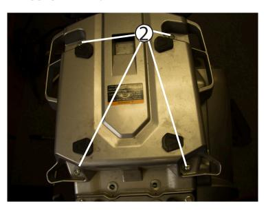
Using a T30 driver remove the (4) OEM M6 screws. Do not remove the washers. Save screws but you will no longer need them for this installation.
