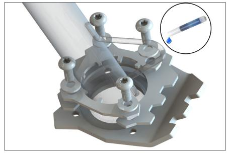
Take the (4) screws and add the washers and a small drop of thread locker to each screw. Now match up the bottom plate to the middle, and top plates and install all (4) screws with washers. Do this in the order shown in the picture.
