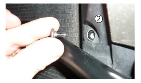
Remove right and left side screw in plastic shroud. TIP! If you have crashbars installed, loosening the crashbars' attachment bolts will allow them to be shifted out of the way and may make installation easier.
