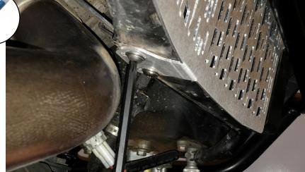
Apply a drop of loctite and attach the two lower M5 x 16 screws, with stainless steel washers under bolt heads, and tighten to 5 Nm. \*\*\*For 1290 Super Adventure, place additional 5mm spacers between radiator guard and radiator mount points.\*\*\*
