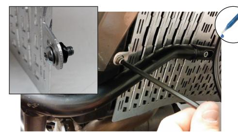
Apply a small drop of loctite to two of the M5x16 button head torx screws. Attach side tabs. Place stainless steel washer between screw head and radiator guard, plastic hat washer fits between radiator guard and black OEM plastic shroud. Tighten to 5 Nm. \*\*\*For 1290 Super Adventure, place tabs behind first layer of black plastic fairing.\*\*\*
