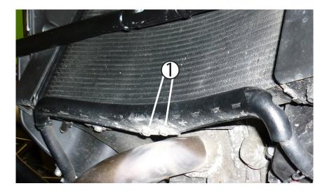
(1) Use T30 torx and remove two screws at center of radiator lower edge.
