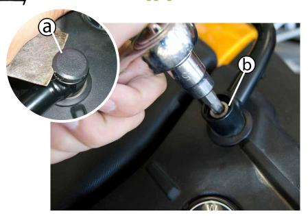
(a) Using a thin flat blade, screwdriver or putty knife, pry out the (2) plastic caps on the grab handle fasteners. (b) Using a T45 torx tool, remove the (2) grab handle fasteners.
