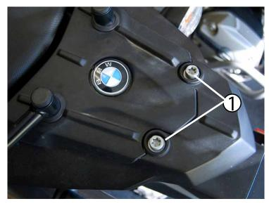
Using a T45 torx tool, remove the (2) rear fasteners indicated.
