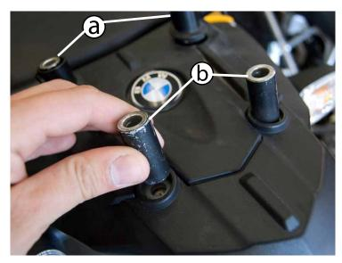
(a) Place the (2) short spacers as shown. (b) Place the (2) long spacers as shown.
