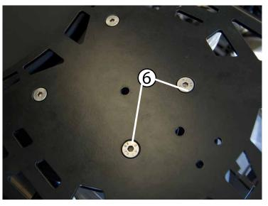
6) Using a 5mm allen tool, tighten the two rear fasteners down.
