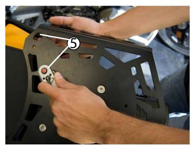
Using a 5mm allen tool, tighten the grab handle fasteners. When tightening these, it may be necessary to pull on the grab handle a little to line up the fastener properly. (my right hand above)
