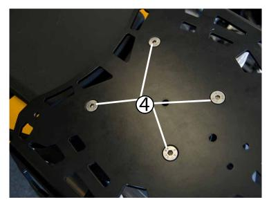
Put all four fasteners in the luggage rack. Line up the fasteners and place the rack as shown.
