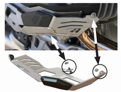
(3) TIP! Note location of 5mm x 5mm spacers, to be installed later. TIP! If you have engine guard bars installed (AltRider or BMW), they will need to be completely loosened up so they can be moved aside in order to install the cylinder head guards. Complete removal should not be necessary, but may make the installation easier.
