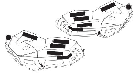
Install five (5) silicone strips and one rubber dome per each left and right guard, in locations as shown above.
