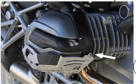
(5) **Right side guard:** Add a drop of thread locker to the BMW screw removed in step 3. Place 5mm x 5mm spacer behind guard and install screw loosely.
