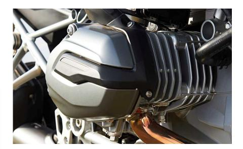
(4) **Right side guard:** Use T25 Torx wrench and remove screw at front of cylinder head that holds plastic cover. Save this screw for reinstallation.
