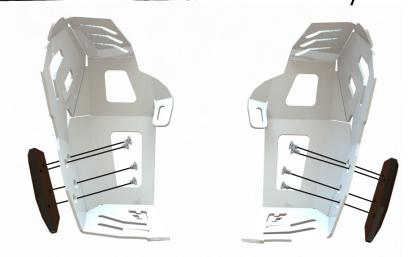
① On each guard, use four M5 x 6mm long flathead screws with thread locker to install the aluminum skid block.
