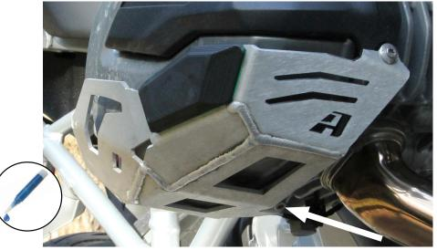
6 **Right side guard:** Add a drop of threadlocker to one of the M5 x 16 button head torx screws that came with the kit. Place 5mm x 5mm spacer between the guard and cylinder head. Place one washer on the screw and install in lower mount hole of guard. **!TIP** It may be necessary to clean dirt out of the threaded hole (with pick and compressed air) in the cylinder first.
