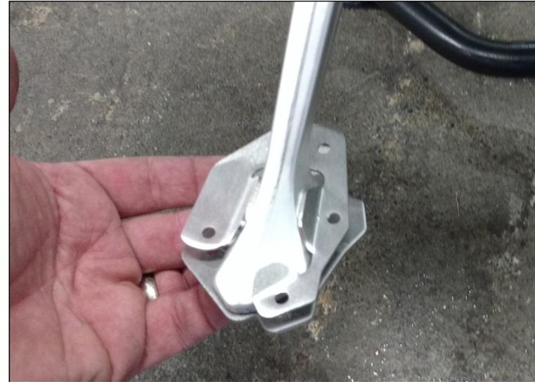
② Position the bottom plate so the holes all line up.
