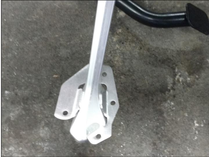
① Slide the top plate over the foot of the side stand as shown.
