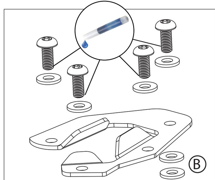
③ Apply one drop of Loctite to the last couple threads on all of the fasteners, then assemble the large sidestand foot on to your sidestand. (B) Be sure to place (2) washers between top and bottom plate.
