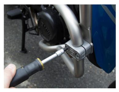
Add the 2nd half of the clamp, (2) washers, and (2) bolts to each side in that order. Tighten with an M5 allen driver so they are snug. Check alignment and then torque all (4) bolts to 9 nm.
