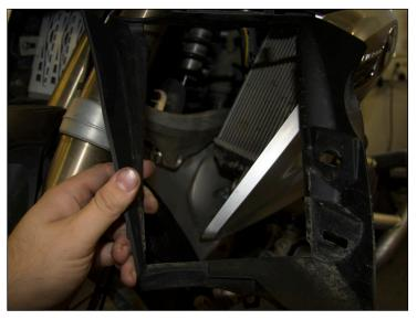
Remove the plastic shroud from both right and left radiators. Be mindful of small male locator pins on the top of each shroud.
