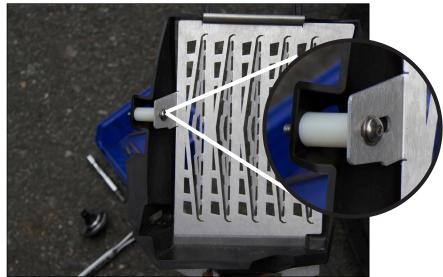
On each side finish assembling the radiator guard to the plastic shroud by installing the M5 x 40mm screw, M5 washer, and spacer to the assembly. Reference photo for correct order. Poke screw through as shown to make installation easier.
