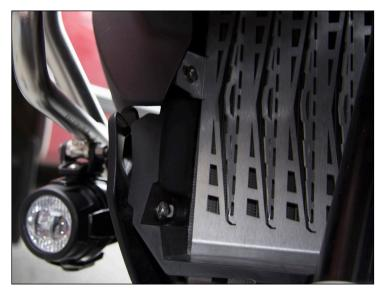
Reinstall the shrouds with the radiator guards installed on them. Start by inserting the locator pins on the top of the radiator shroud. Reinstall the (2) OEM screws on each side and tighten. Also tighten the (1) M5 screw using a 3mm allen.
