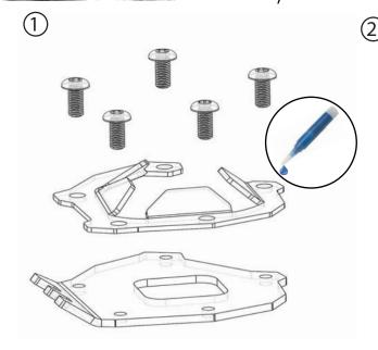
Add thread locker to the tip area of each screw. Arrange side stand foot in place. Start the two screws closest to the bike (at the tips of the upper plate) by hand. Then place and start the rest of the screws but do not fully tighten yet.
