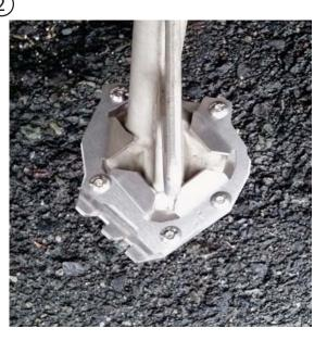
Snug each screw tight in turn. These should be just tight enough that the tips of the screws sit flush with the underside of the bottom plate. There will still be a gap between the plates when installation is finished.
