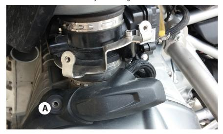
Install left bracket as shown. Each hole has M5 x 35 screw, two washers (one top and one bottom), and M5 lock nut. Tighten screws. Remove front OEM T25 Torx from plastic cover. (A) You will not re-use this screw.
