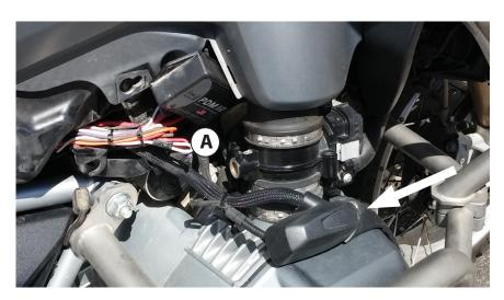
Clip small zip tie (A) at location shown to free up hole. Remove OEM M5 screw with T25 Torx at front of plastic cover, you will not reuse this screw. (arrow)
