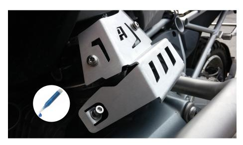
Place 16mm long spacer behind front mount location. Put drop of threadlocker on M5 x 35 screw and screw in with washer. Tighten all screws. Reinstall side plastic cover. (Screw with longer shoulder goes through double layer of body panels.)
