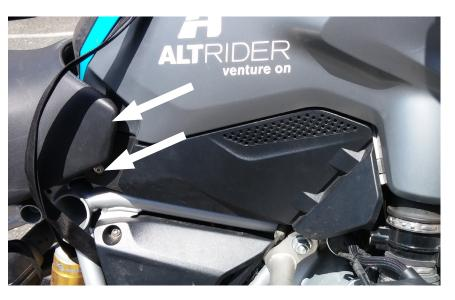
**Right side guard:** Remove black plastic fairing by removing two T25 screws under front edge of seat. Keep these screws and note length for re-installation later. Gently slide fairing rearward to remove.
