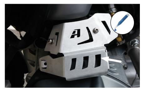
Place aluminum cover in location. Put a drop of thread locker on two M5 Torx screws, put a washer on each screw, and install loosely to bracket.
