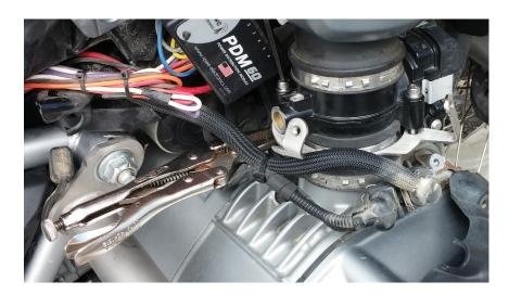
Install right side bracket as shown. Each hole has M5 x 35 screw, two washers (one top and one bottom), and M5 lock nut. Tighten screws. Use needle-nose vise grips to hold nut and get started on rear screw, then 8mm combination wrench to tighten.
