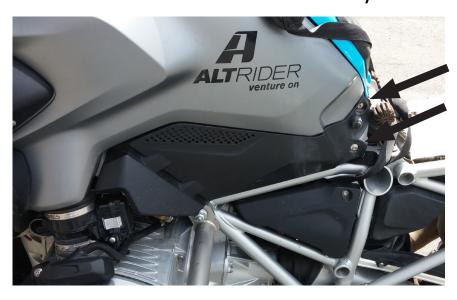
Left side guard: Remove black plastic fairing by removing two T25 screws under front edge of seat. Keep these screws and note length for re-installation later. Gently slide fairing rearward to remove.
