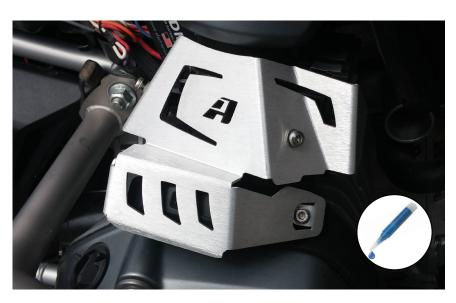
Place 16mm long spacer behind front mount location. Put drop of threadlocker on M5 x 35 screw and screw in with washer. Tighten all screws. Reinstall side plastic cover. (Screw with longer shoulder goes through double layer of body panels.)
