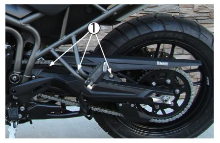
Use a 5mm allen tool to remove the (3) OEM button head fasteners.
