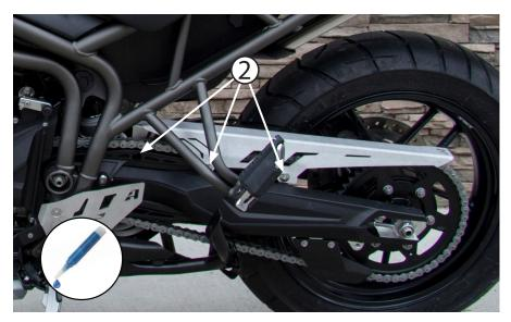
2 Apply a drop or two of thread locker to the end of each of the OEM button head fasteners. Use the 5mm allen tool to attach the AltRider guard to the (3) OEM mount tabs. Tighten all (3) OEM button head fasteners.
