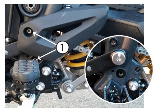
Use a 5mm hex tool to Remove the (2) M8 button head fasteners from the OEM heel guard and remove the guard. You may need to remove the rubber foot peg pad in order to remove the lower bolt.
