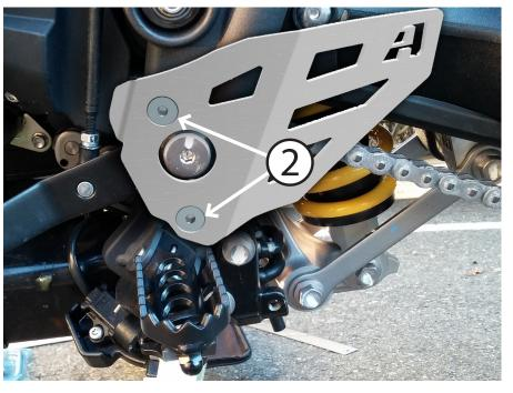
Apply two drops of thread-locker to the ends of the (2) M8 flat head fasteners provided. Install the new guard with the spacers positioned on the M8 flat heads, BEHIND the guard.
