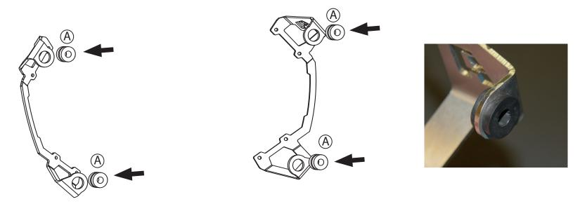
Install four (4)rubber grommets into headlight guard. (A) Use care to not rip the rubber. **!TIP** a dab of water will help them slide into place, a small flathead screwdriver is a good tool to use.
