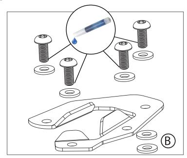
Apply one drop of Loctite to the last couple threads on all of the fasteners, then assemble the large sidestand foot on to your sidestand. (B) Be sure to place (2) washers between top and bottom plate.
