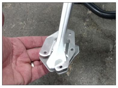
(7) Position the bottom plate so the holes all line up.
