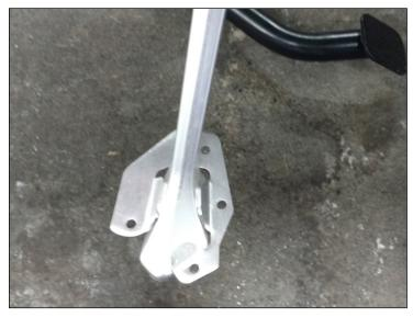
(1) Slide the top plate over the foot of the side stand as shown.
