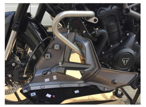
"Thread" the upper mount flange of one side crash bar through the bottom opening in the fairing. You can now let the fairing hang as shown while you complete the install. Do this for both sides.
