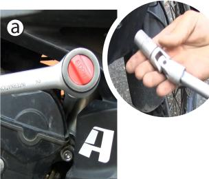
Remove the 2 upper M10 engine bolts using an extension, universal joint and M14 socket reach behind the frame (a) then use an M8 allen key (or T50 Torx, 2014 and on) (b) to hold and remove. Be careful to capture nut when it comes loose. You will re-use the left side bolt but not the right side bolt.
