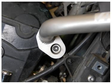
Install the AltRider provided M10 x 70mm socket head cap bolt (using the OEM nut) but do not tighten all the way.
