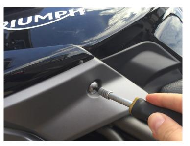
6 Use a 5mm allen tool to remove the single button head fastener on the exterior of the fairing.
