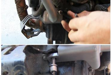
Install left bar by sliding the lower flange in front of coolant hose. Start the OEM Hex (socket cap shown) bolts but do not tighten completely.
