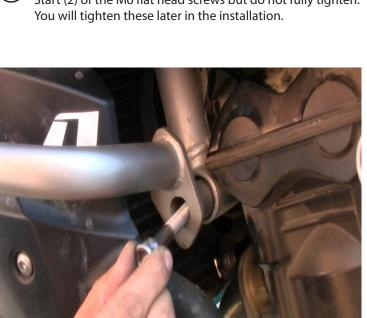
Reinstall the OEM M10 engine bolt + nut without washer but do not tighten completely.
