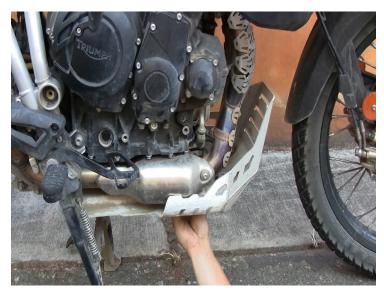
If OEM or after market skid plate is installed remove this now. On XCX models, remove OEM crash bars.
