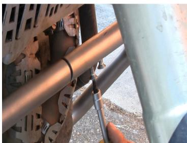
Now go back and tighten all (4) M6 x 20 flat head screws holding the center connector and both bars sides in place. Tighten each screw to 8nm of torque by alternating from one screw to another so they tighten evenly.
