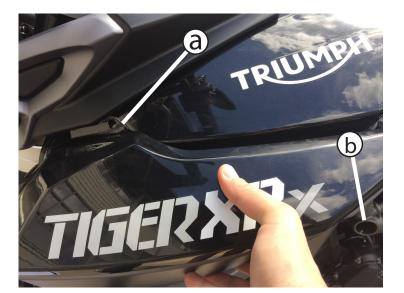
[a] Gently replace the fairing, ensure it seats in the (2) rubber grommets then [b] use a 5mm allen tool to replace the fastener.
