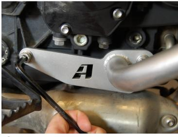
Start (2) M8 socket cap screws on lower right side mount, do not tighten all the way.
