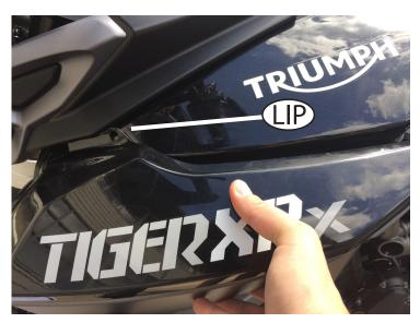
Gently lift the fairing, dislodging it from the (2) rubber grommets then rotate the bottom out so the upper fairing lip can exit the body work. Follow these steps on the other side.
