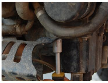
Using a 12mm socket, remove hex bolt on left side directly underneath the oil filter. Save this bolt but you will need it later in the installation.
