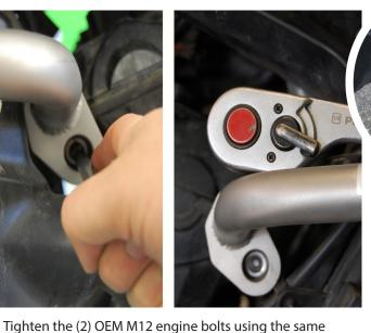
Place a dab of grease inside of your socket to keep the nut from easily falling out.
