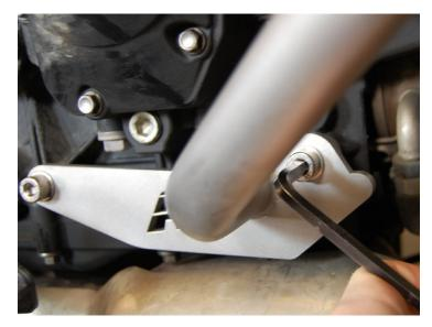
Tighten all (4) lower mount bolts to 20nm of torque. There are (2) bolts on each side.
