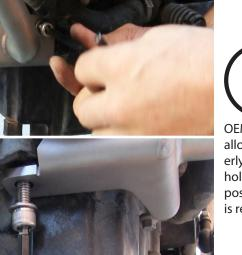
OEM bracket may not allow lower bolt to properly align and sometimes holding the bar or repositioning the bracket is required.
