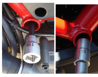
Using an 8mm allen key on one side and a 15mm socket on the other, remove the motor mount through bolt.
