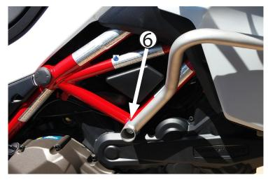
(a) Insert one M12 washer into the frame socket.
