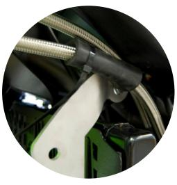
Take the rubber tube provided and use scissors to split it. Wrap it around the stainless oil line and zip-tie it in place as shown above. (AltRider bracket shown in pic above, but easier to install the rubber tube now before bracket in place)
