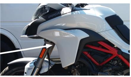
(7) Oil lines are located above front left corner of radiator.
