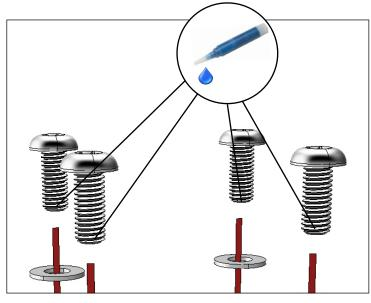
Apply one drop of Loctite to the last couple threads on all of the fasteners, then assemble the large sidestand foot on to your sidestand (indicated in step2). For Multistrada 950, do not install the washers.
