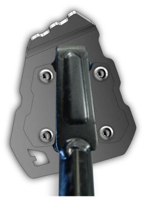
2 Looking down on the top of the large sidestand foot assembly, place the foot so that it is aligned as shown. Once in place, tighten all of the fasteners.
