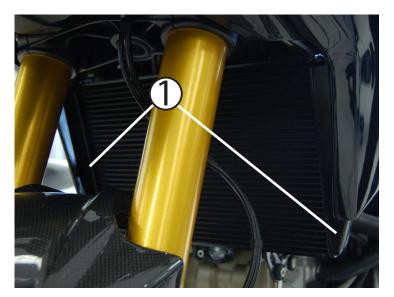
Ensure the radiator is cool to the touch before beginning. Lightly abrade paint at tape locations with scotchbrite pad. All that is necessary is that the glossy surface be lightly scratched. This will ensure the optimum bond. Using the provided isopropyl alcohol wipe clean both ends of the radiator, then ensure they are dry before proceeding.
