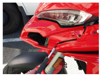
(1) Using a 3mm allen tool, reinstall the (4) screws ((2) right and (2) left) that secure the beak to the rest of the fairing.
