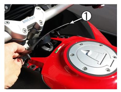
① Remove the small black plastic cover surrounding the ignition switch (what used to be the key hole).
