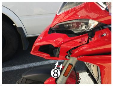
Practice inserting the oil cooler guard from below, you should have just enough clearance with the beak pulled out and tilted up slightly. Once you are confident with your placement, pull the guard out and peel off the backing from the VHB tape, insert from below and apply pressure to secure it.
