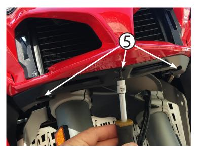
(5) Using a 3mm allen tool, remove the (3) fasteners under the beak. Note: you may need to rotate the fork for best tool access.
