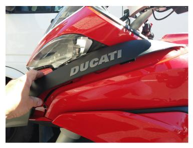
(12) Reinstall black plastic "spears" Note there are 3 tabs/slots to line up. One at the very front near the nose openings, two on the side. Place in location and slide rearward with hand pressure.
