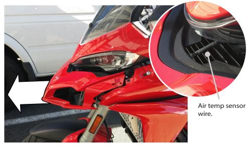
Slide the entire beak forward about 1.5". Do not slide too far! There is a temp sensor wired from the main body to the beak, be careful not to damage this wire.
