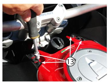
(13) Using a 3mm allen, reinstall all (4) of the fasteners indicated.
