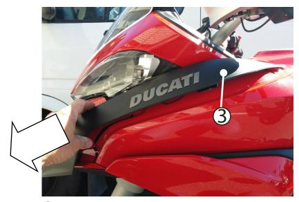
3 Remove the black plastic trim pieces on either side of the fairing. Use two handed pressure and slide the pieces forward to disengage the mounting tabs/slots.
