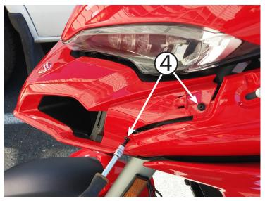
Using a 3mm allen tool, remove the two screws on each side (4) in total. Note that these fasteners have small plastic washers on them, be sure to not lose any.
