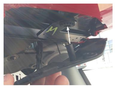
Using a 3mm allen tool, reinstall the black under-nose piece (3 screws).
