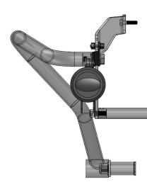
3 Adjust both brackets to same level, tighten all mounting bolts.
