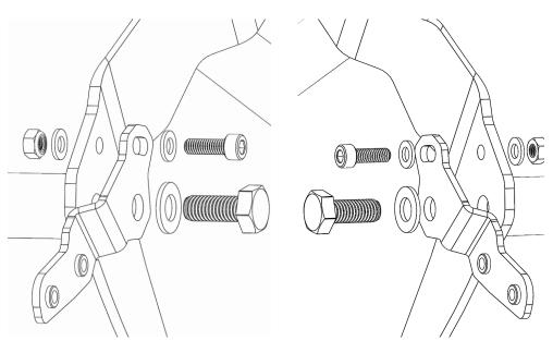
Attach LED brackets as shown. Place LED bracket against inside surface of the crashbar brackets, re-insert M10 hex bolt. Insert M6 screw, washers, and lock nut as shown. Note brackets should bend outward from centerline.
