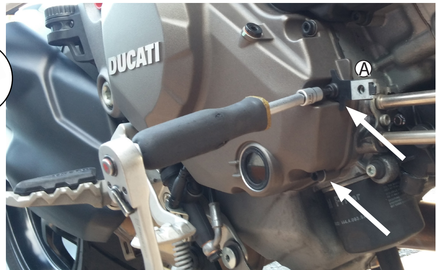
④ 5mm allen wrench, remove 2 screws shown, remove small black bracket (A)
