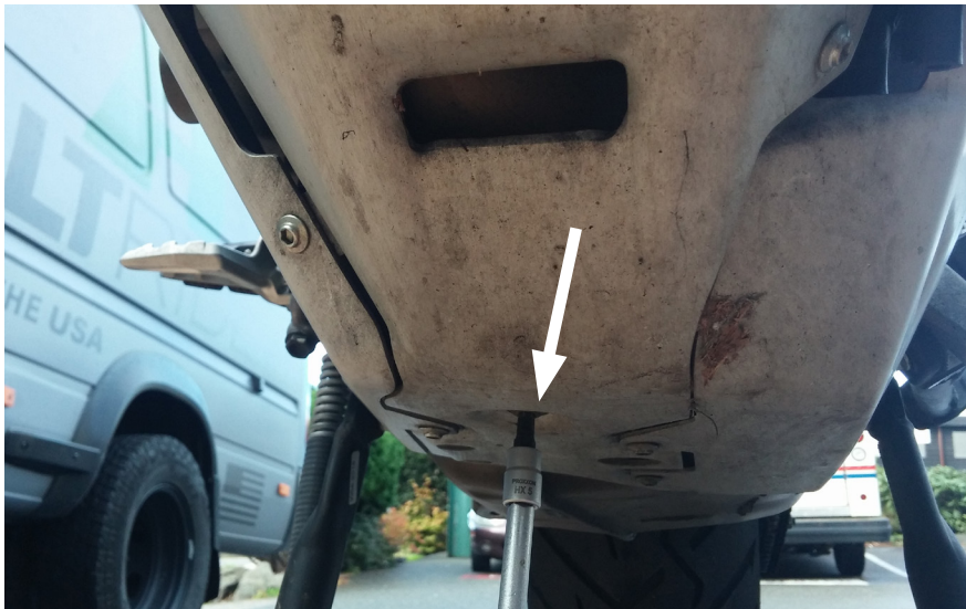
③ Remove bottom screw, M6 allen wrench.
