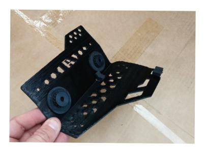
Install rubber bushings as shown, through large washers and AltRider guard. Use small bit of water to lubricate and help get in place, careful not to tear. Be sure bushings are fully seated both sides. Install internal metal spacers.
