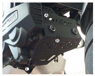
Install AltRider guard using all OEM hardware. Clip plug into small rectangle hole provided.(A) Use cable tie to secure plug and wiring behind guard,(B) be sure not to pinch the wires. Install rubber loop at lower edge to capture wires (C). Torque screws to 2.7 Nm.
