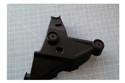
Remove OEM guard. Clip zip tie on rear, remove small rubber loop at lower edge. Remove internal metal spacers and remove rubber bushings.
