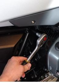
① Use 18mm socket and T55 torx to remove the engine through bolt. You will not reinstall this bolt.
