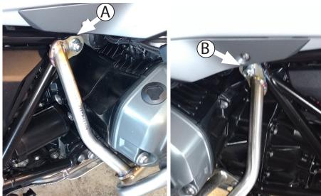
(A) Insert AltRider through bolt through the right hand reinforcement bar, then through the engine.
