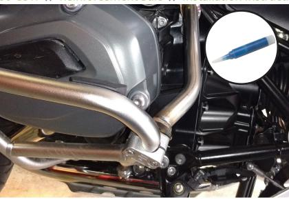
Visually align reinforcement bar with through bolt location but attach the clamps to the left and right side first, don't tighten all the way. Add a drop of thread locker to the tip of each screw. Insert M6 x 35 screw with washer through both clamp halves and into the threaded hole in the tube flange.
