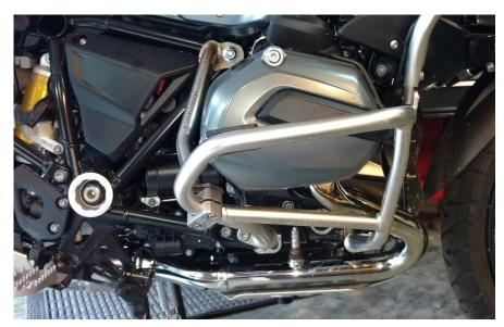
Adjust the bar location for good fit. Tighten the the M12 nut to 85Nm first then M6 screws to 7.5Nm.
