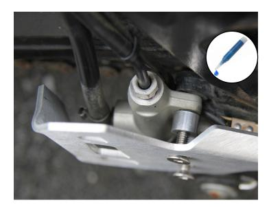
Install AltRider guard with (2) provided M6 screws and (2) custom spacers. Stack the guard, spacers, and screws as shown above. Use thread locker on both screws,
