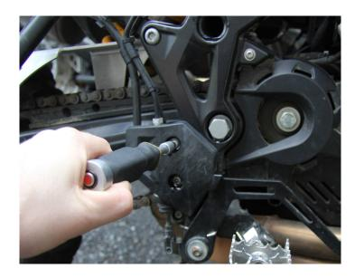
Using a T30 Torx driver, remove the (2) OEM M6 screws and OEM guard.
