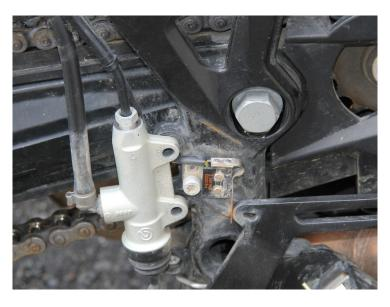
If there is excessive dirt, grime, rocks, or other debris, now is a good time to remove them. Also make sure that your sensor and connections are all in good shape. Also check the condition of your master cylinder.
