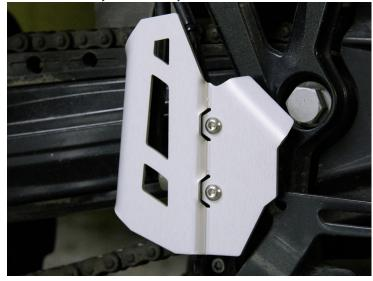
Tighten both M6 screws using an M4 allen driver. Torque both to 10nm of torque.
