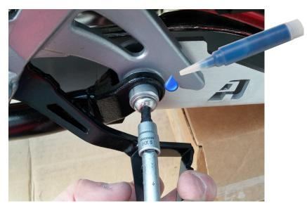
With bike still on side stand. Apply loctite to each M8 x 45mm long Button Head bolt. Install bolt with washer through each hollow center stand pin and into the threaded insert in the skid plate. Tighten each M8 bolt to 10nm of torque.
