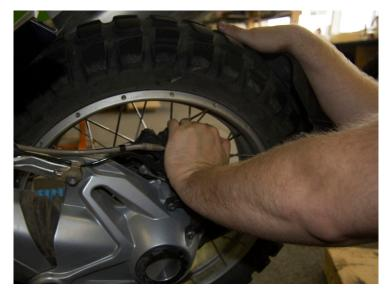
Place the bike on its side stand. Using your hand compress the rear brake caliper so you can freely move the rear brake lever down.
