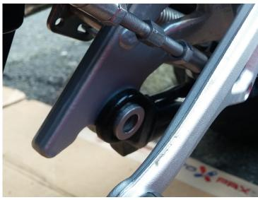
6 Adjust pins so they are centered on the frame, with a few millimeters protruding from both the inner and outer side of the center stand pivot.
