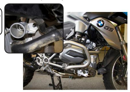
Remove the (2) OEM M10 bolts from frame spar (refer to step 3 for example image). Hang right side crash bars and begin to thread the 2nd M12 nut to hold bars hanging in place. NOTE: front upper mount should be positioned inside the frame.
