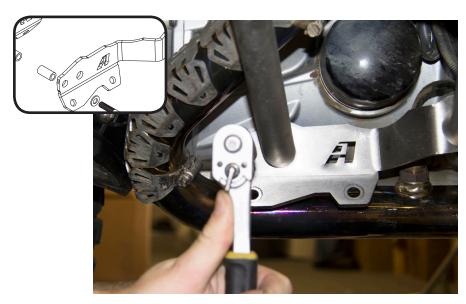
(6) Install the M8 x 50mm bolt with washer, and spacer into the front mount position of the lower bracket. Use anti-seize. Do not torque all the way.
