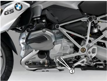
Using a T50 driver remove the (2) OEM M10 lower engine mount bolts on the left side.
