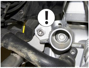
Install the (1) M8 bolt, (2)washers, and (1)lock nut to the top front mount using an M6 driver and 13mm wrench. The crash bar mount should be situated on the inside of the bike frame.
