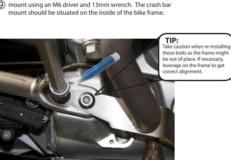
Reinstall the (2) OEM M10 bolts using a T50 driver and clean bolt threads, chase threads in engine, apply thread locker, reinstall and do not tighten all the way. Go back to the front and upper M8 bolts in step 9 and 10 and torque to 10 nm or torque. Return to the (2) OEM M10 bolts and torque to 55 nm or torque.
