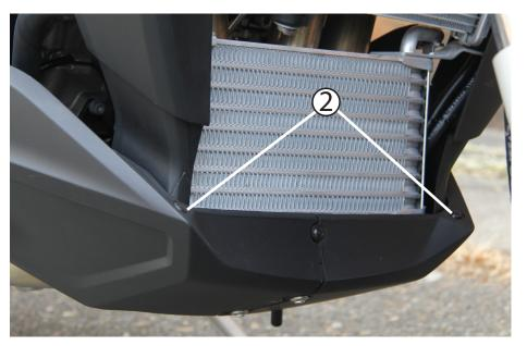
Use a thin tool (a 3mm allen tool or t-8 torx tool will work) to push the centers of the plastic toggle clips through. Pay attention to where they go, they have a tendancy to shoot out. Remove only the front left and right corner toggles, no need to remove the center one. You can now remove the lower fairing and set it aside.
