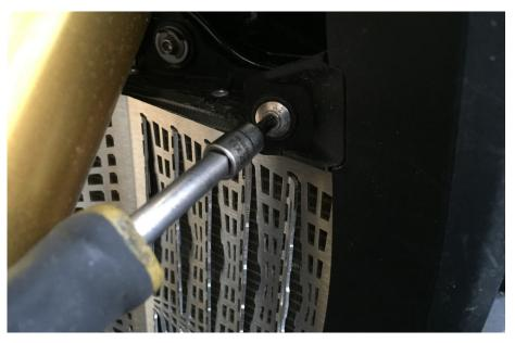
Place the radiator guard over the radiator but underneath the rubber grommets of the plastic fairing tabs, get (1) of the OEM fasteners started and then the other, do not tighten them down yet.
