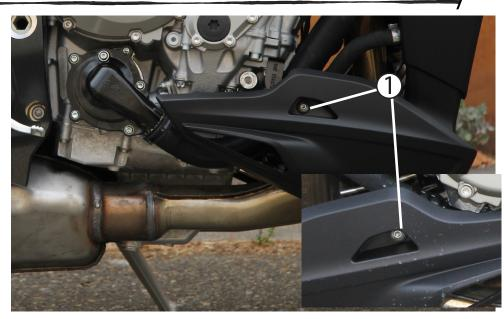
Use a T-25 torx tool to remove the (2) OEM lower fairing fasteners on the left and right of the lower fairing.
