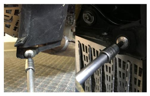
Using a t-25 tool, go back around to each of the mounting points and tighten them, making certain that everything lines up correctly before tightening all the way. Replace the lower plastic fairing and you are ready to ride.
