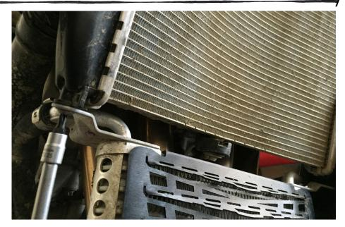
Flex the plastic fairing out, you can now see the lower mount tabs for the oil cooler. Using the t-25 tool, remove the (2) OEM lower mounting fasteners (without shoulders) which attach the oil cooler to the radiator.
