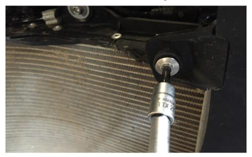
Using a t-25 torx tool, remove the upper (2) OEM fasteners (with shoulders) as well.
