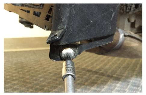
Using a t-25 torx tool, remove the (2) OEM fasteners holding the bottom of the plastic fairing to the oil cooler, note the long shoulder on these fasteners, they are meant to be used with the thick rubber grommets.
