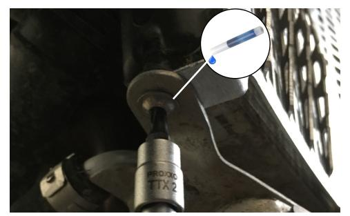
Stack the oil cooler mounting tabs over the radiator guards' mounting tabs. After applying a drop of thread locker to the last couple of threads of each OEM fastener (with no shoulder) Use a t-25 tighten these (2) fasteners all the way.
