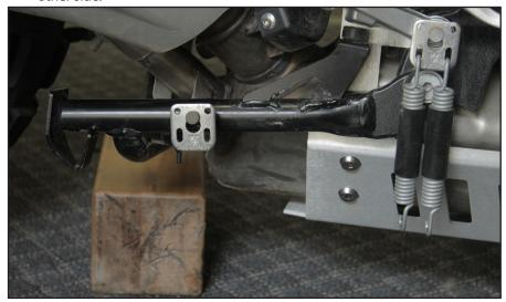
Now tighten each of the fasteners down starting with the flat head M6s which you can tighten until snug. Finish with the main mounting brackets' M10s, tighten to 40nm. Tighten the M8s the t40s and the center stand pin to 25nm. Take the bike off of the center stand and put it back on the side stand. Use a block of wood to prop the center stand up to assist with installing the springs.
