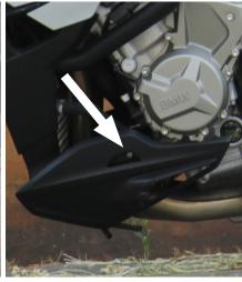
3 Use a T25 torx bit and remove the two screws (one right side, one left) that attach the lower fairing. Save these for reinstallation. Remove the fairing and locate small plastic pins from step 2. Save all for reinstallation.
