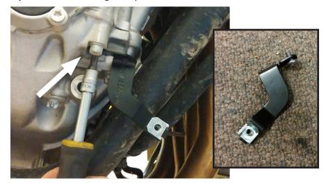
Use a T-30 torx tool to remove the right side bracket that holds the lower fairing, you will not reuse these parts.
