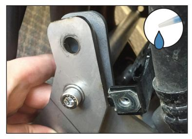
8 Now on the left side position the front left skid plate bracket as shown, and (A) insert the M8 x 35 fastener with M8 washer as shown. (B) Next insert the M8 x 25 fastener with M8 washer as shown, do not tighten all the way yet.
