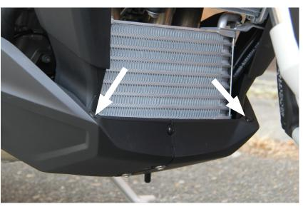
Remove plastic lower fairing. Start by detaching the small plastic rivet at each front corner. Push the small central pin inward. Caution, watch where it goes inside the fairing! Then pull the head of the plastic rivet outwards. Save these parts and store them with the plastic lower fairing, you will not be re-using these parts.
