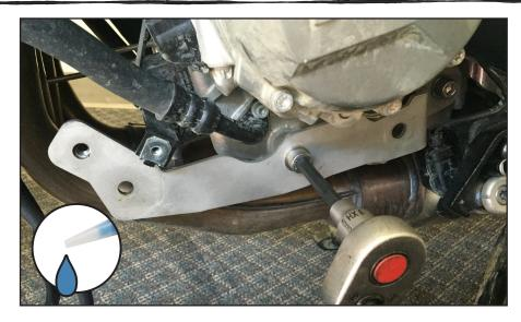
Start with the left side mounting bracket and align as shown. After applying blue thread locker to the last couple of threads on each of the (2) M10 x 20 fasteners with M10 washers, use a 8mm allen tool to attach the bracket to the bike as shown. Do not tighten the fasteners all the way down, leave the bracket loose so that you can adjust it.
