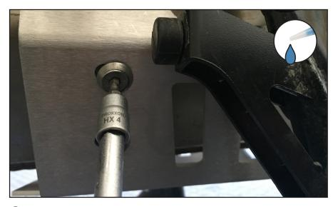
13 Now that all of the brackets are in place, hold your skid plate up and get a sense of how it will be fastened. It is recommended to start with the rear brackets. After applying thread locker to them, use a 4mm allen tool to get the (2) M6 x 15 flat head fastener with finishing washer started on one side. Leave them loose as you have on all the other fasteners. Now do the other side.
