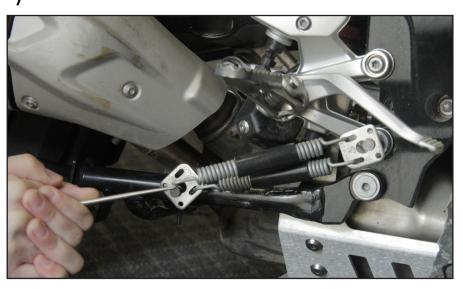
Place your bike on its side stand temporarily. Use a spring-puller to release the center stand return springs, do them one at a time. Put the bike back up on the center stand. Verify the bike is stable, do not do this step on an incline.
