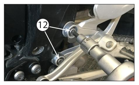
On the left side of the bike, use a T45 torx tool to remove the (2) OEM bolts from the left rearset. Align the left rear skid plate bracket as shown and reinsert the (2) OEM bolts as shown, leave loose for now.
