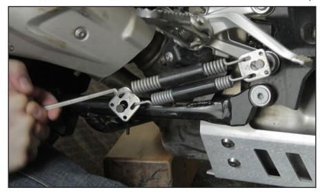
Place the spring hanger plate back on the pin and hang the springs. Using the spring puller tool, pull one spring and then another and hook them on to the plate as shown. The wood block holds the stand up so that you pull backward, instead of down which has limited space.
