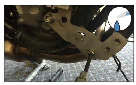
Install the mounting bracket cross-tube. Apply thread locker to each fastener. Each side uses one M8 x 35 socket cap bolt. Attach the right side first, but leave it loose, do not tighten all the way yet.
