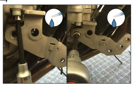
The right side mounting bracket will essentially take the place of the OEM bracket you removed in step 4. **(A)** After applying thread locker to the fasteners, use a 5mm allen tool to get the (1) M6 x 16 bolt and M6 washer started first, do not tighten it down yet. **(B)** Next, using a 6mm allen tool, get the (1) M10 x 20 bolt with M10 washer started in the location shown. Do not tighten all the way yet.
