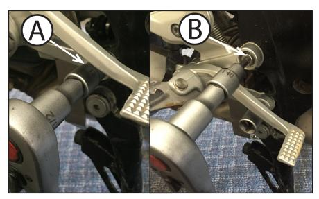
(A) Using a 15mm socket, remove the pin which the springs were attached to, you will be reusing this pin so keep it close. (B) Next use a T45 torx tool to remove the upper bolt as shown. Place the right rear skid plate bracket as shown and use the (2) OEM bolts you just removed to secure it, leave loose for now.
