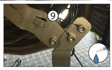
Position the right front skid plate bracket as shown. After applying thread locker to both fasteners, use a 6mm allen tool to install the (2) M8 x 25 fasteners with washers as shown. Do not tighten all the way yet, you want the bracket to have a generous amount of adjustability.
