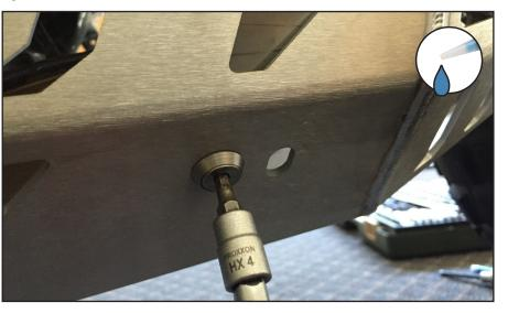
The skid plate should be hanging in place at this point. Use your 4mm allen tool to continue to install the front (4) M6 x 15 flat head fasteners with finishing washers on the left and right front skid plate brackets to finish attaching the skid plate. You may need to move the front right or left brackets a little by hand to get the holes to line up properly. Once you have all (8) OEM fasteners {(4) in front and (4) in the rear} started move on to step
