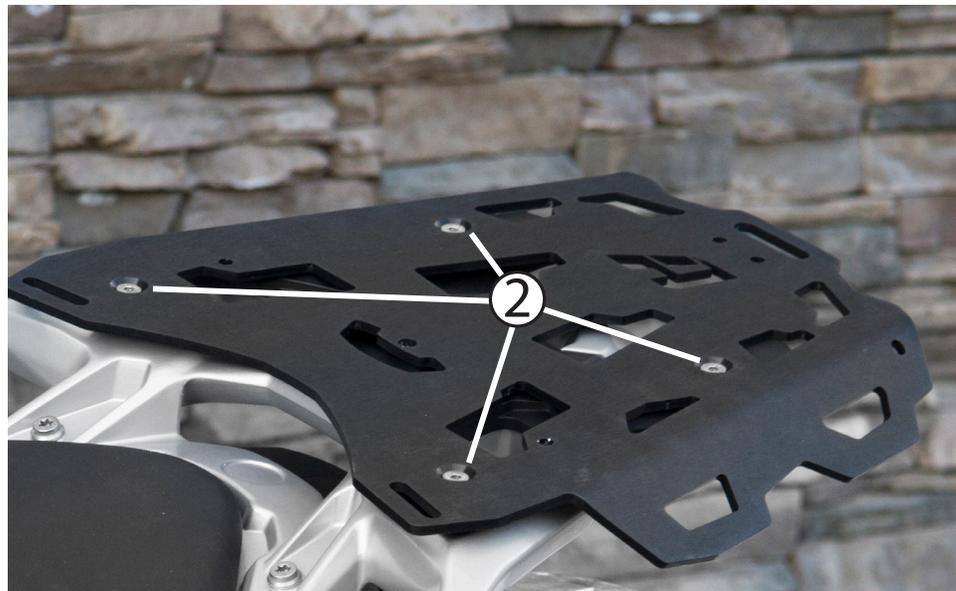
② Insert the (4) M6x25 Flat Head fasteners and use a 4mm allen tool to tighten them to 26.5lbs (3nm).
