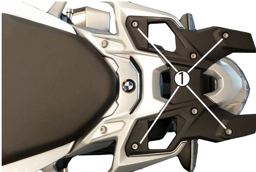
① Use a T-30 torx tool to remove the (4) OEM fasteners.
