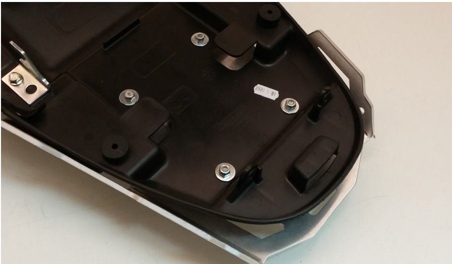
③ Place one washer and one lock nut on each screw. Attach loosely, do not tighten fully.
