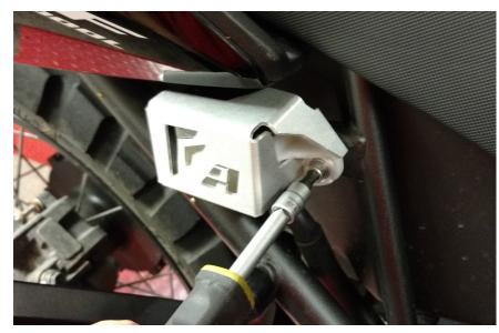
3 Use 4mm allen tool with M6 cap head screw and washer to reinstall the reservoir guard.
