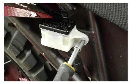
Use 8mm socket to remove the screw holding the rear brake reservoir in place.
