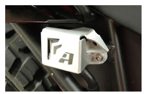
After 5 hours of riding, or 100 miles, check all the fasteners on the assembly to ensure they are tightened to spec.
