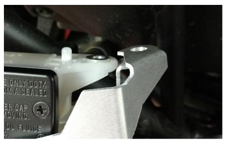
2 Slip the AltRider reservoir guard in place, with one mounting tab on the outside and one behind.
