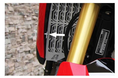
Insert the spacer behind the small tab and insert the M5 button head screw with washer and screw tight. Finish tightening both M8 bolts from step 3.
