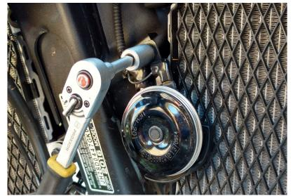
For left side guard, first use 12mm socket to remove the horn with it's mounting tab.
