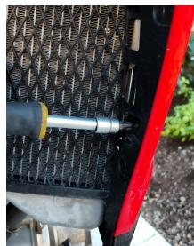
Remove two phillips screws in inner shrouds (one on left side, one on right side). You will not re-use these.
