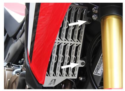
(3) Install right side guard as shown. Start by getting the two M8 bolts with washers started loosely through the AltRider radiator guard.
