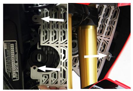
Install left side guard as shown. Start by getting the two M8 bolts with washers started loosely through the AltRider radiator guard. Insert the spacer behind the small tab and insert the M5 button head screw with washer and screw tight. Finish tightening both M8 bolts.
