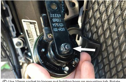
6 Use 10mm socket to loosen nut holding horn on mounting tab. Rotate horn so that the wires line up with mounting tab as shown. Tighten nut.
