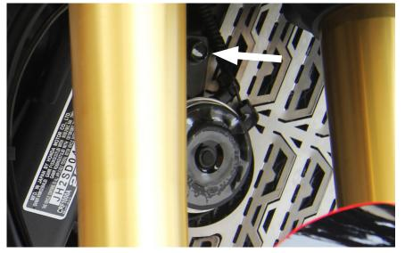
(S) Use 12mm socket to reinstall horn with OEM bolt.
