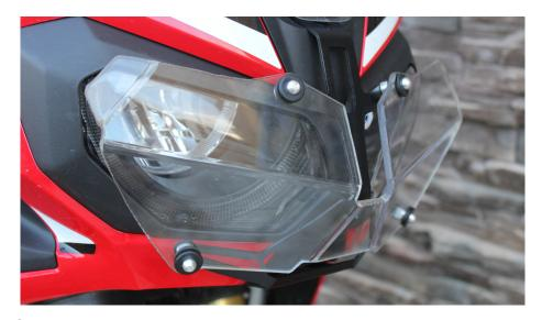
Install headlight guard. **!TIP** A dab of water on each ball stud will help it fit in place easier with less wear on the rubber grommets.
