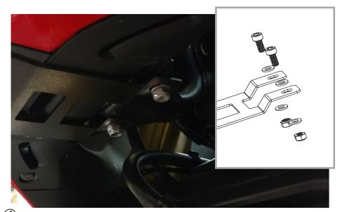
Use (2 qty) M6 x 14mm socket cap screws, (4 qty) M6 washers, and (2 qty) M6 lock nuts to loosely attach bracket to the mounting points under the nose of the bike, as shown.
