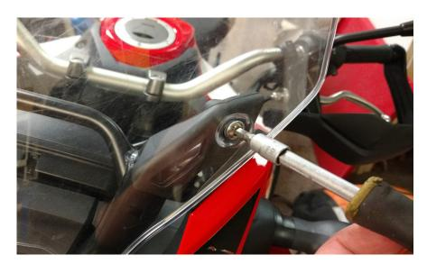
③ Use 5mm allen tool and remove four(4) windscreen screws. Remove windscreen. Save these for reinstallation. **!TIP!** Make sure all four OEM rubber well nuts remain securely in place.
