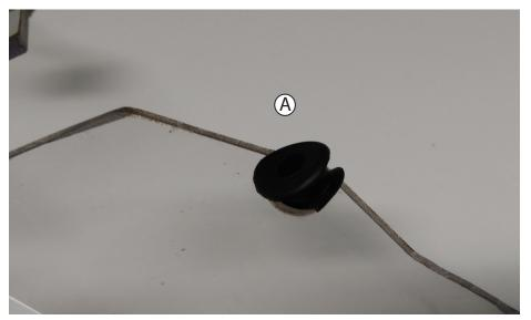
Install four (4)rubber grommets into headlight guard. (A) Use care to not rip the rubber. **!TIP** a dab of water will help them slide into place, a small flathead screwdriver is a good tool to use.
