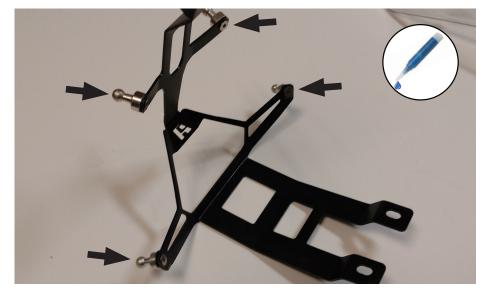
Attach (4 qty) ball studs to bracket with (4 qty) M4 flat head screws. Apply a drop of thread locker to each screw. Use 10mm open end wrench and 2.5mm allen to tighten to 2.3 Nm.
